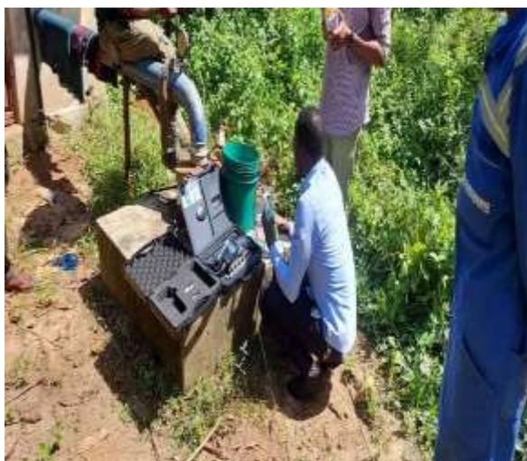
**Plate No. 4.1-1: In-situ Water Quality Examination for Shakanii Drilled Well.**
